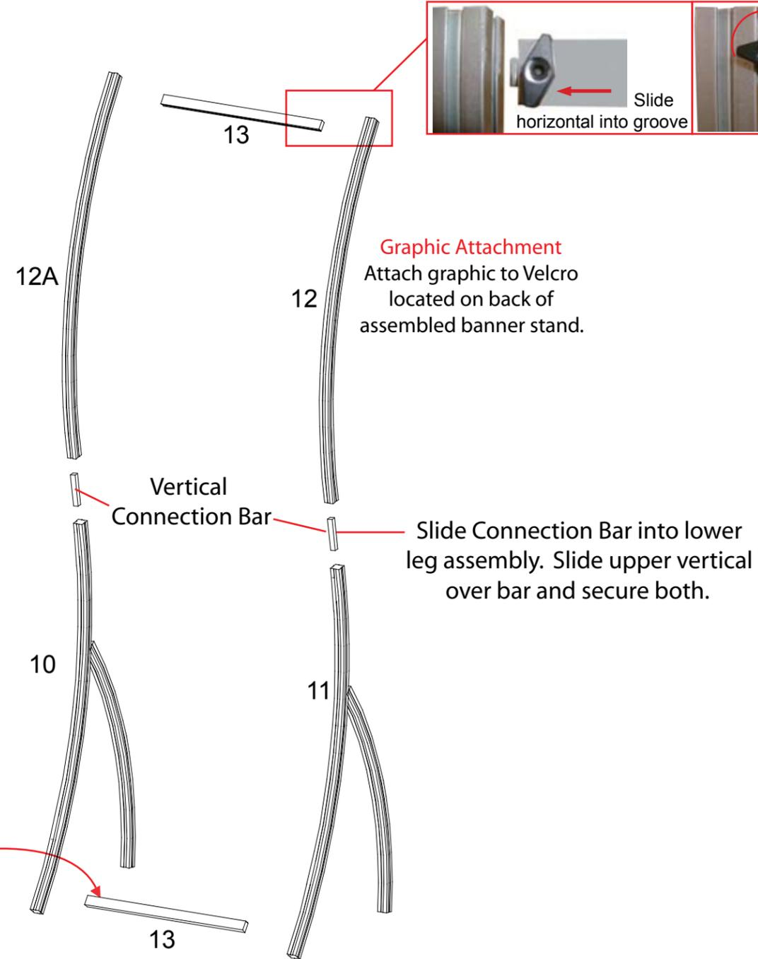
NOTE: When assembling horizontals they should be placed approximately one inch from TOP and BOTTOM.
