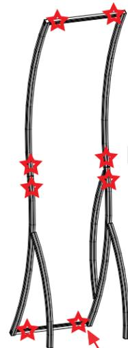
STAR indicates location of knobs on BACKSIDE of unit.
