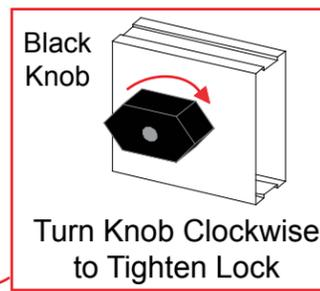
Turn Knob Clockwise to Tighten Lock
